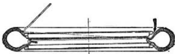
16. Rim and tyre — sectional view — tyre fitting
