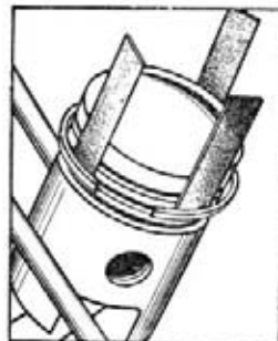
32. Replacing the piston rings
